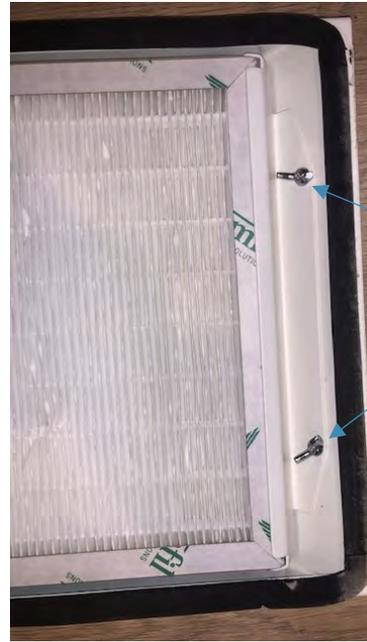
Wing nuts holding filter brace
