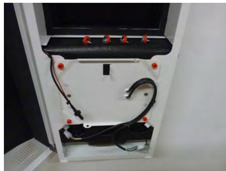
Figure 14 Fan assembly wires unclipped
